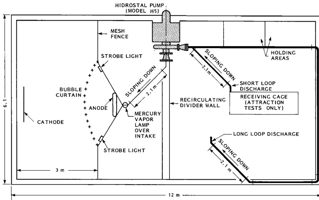
Figure 1. General layout of Hidrostral pump test pool.
