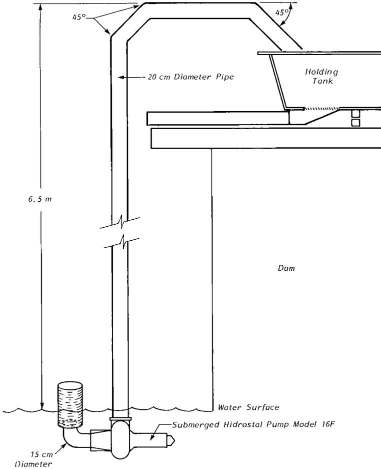
FIGURE 1.—General layout of the Hidrostral pump and transport system tested with American eels at the Saunders hydroelectric facility on the St. Lawrence River.
